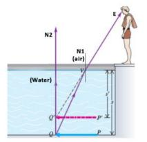
Light coming from the bottom of the pool (let us take a point Q) bends away from normal (N1) at point 'v'. Again light coming from the point Q striking the surface of water perpendicularly (N2) goes out without deviation. If the ray VE, is extended backwards it meets the other ray from Q at Q'. Thus Q' is the image of Q. For the observer the apparent depth of the pool becomes S'— which is less than the real depth of the pool S.
