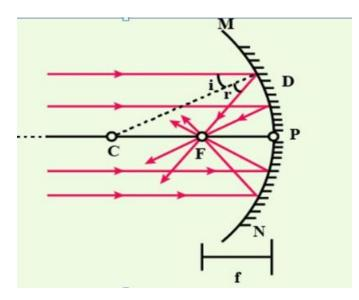
8. Concave mirrors are mirrors that curve inwards, while convex mirrors are mirrors that curve outwards. Concave mirrors reflect light rays inwards, causing them to converge, while convex mirrors reflect light rays outwards,
